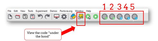
Fig. 7.6: Buttons for running an online study from the PsychoPy Builder. From left to right 1) Run study in browser directly (not project status must be "running", not "piloting" or "inactive"). 2) Sync project/create project on 3) Browse existing projects shared by others on 3) Check what account you are signed in on 4) Project information (note this will only be populated if the currently opened psyexp file has been synced to pavlovia.org)
